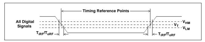
Figure 34 - Timing Parameter Measurement Digital Voltage Levels
