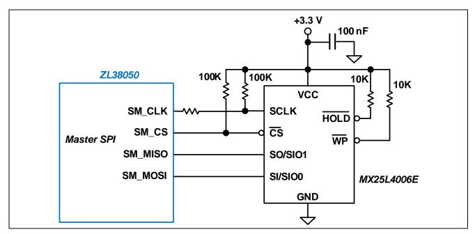
Figure 23 - Flash Interface Circuit
