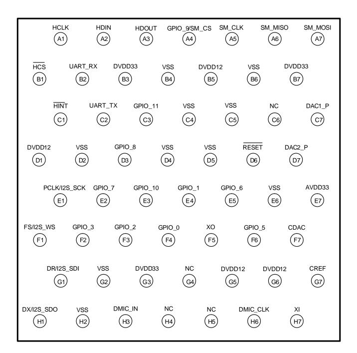
Figure 28 - ZL38050 56-Ball WLCSP - Top View
