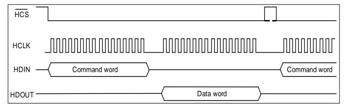
Figure 22 - SPI Slave Command Framing Mode - Read
