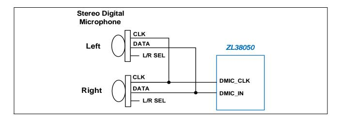
Figure 4 - Dual Microphone or Stereo Digital Microphone Interface
