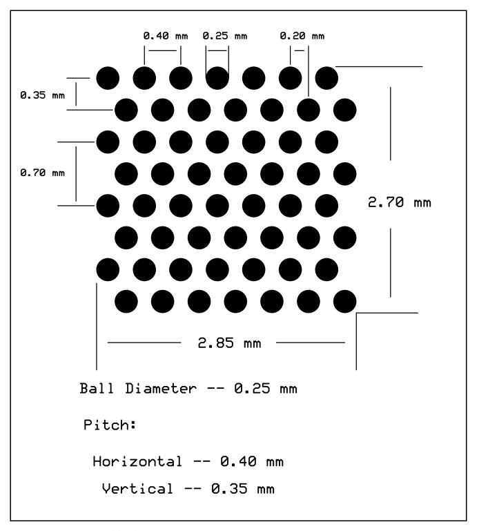
Figure 49 - 56-Ball WLCSP Staggered Balls Expanded Bottom View
