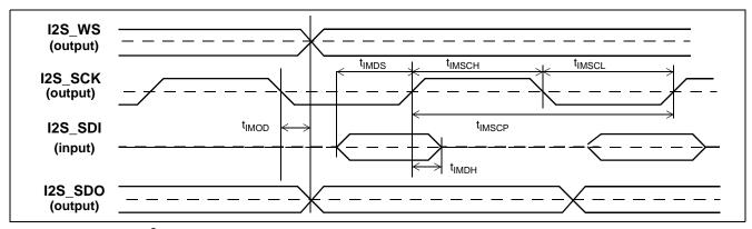
Figure 39 - Master I<sup>2</sup>S Timing
