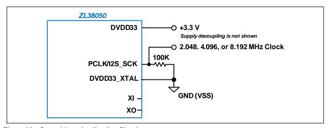
Figure 33 - Crystal-less Application Circuit
