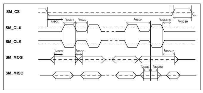
Figure 44 - Master SPI Timing
