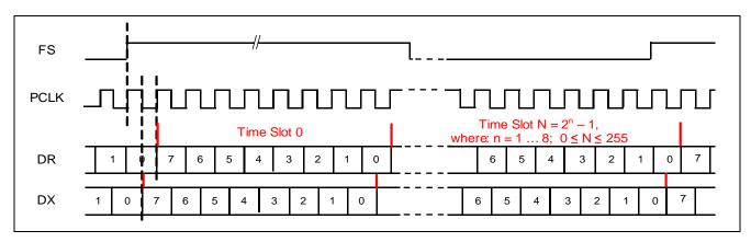
Figure 11 - TDM - PCM Slave Functional Timing Diagram (8-bit, xeDX = 0)
