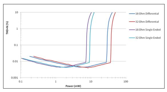
Figure 29 - THD+N Ratio versus Output Power - Driving Low Impedance
