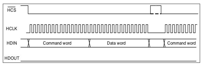
Figure 21 - SPI Slave Command Framing Mode - Write
