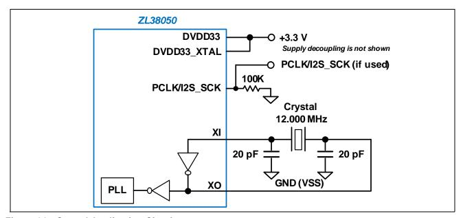
Figure 31 - Crystal Application Circuit
