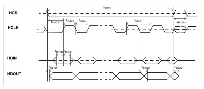
Figure 40 - SPI Slave Timing
