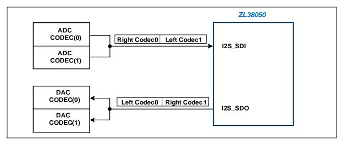
Figure 10 - Dual Codec Configuration
