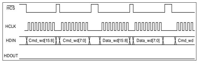
Figure 17 - SPI Slave Byte Framing Mode - Write
