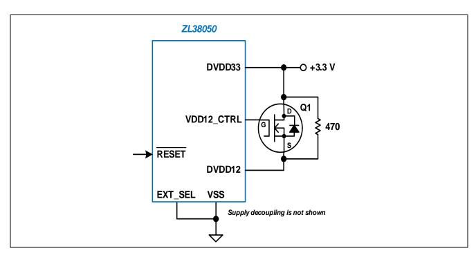
Figure 25 - Internal +1.2 V Power Supply Configuration
