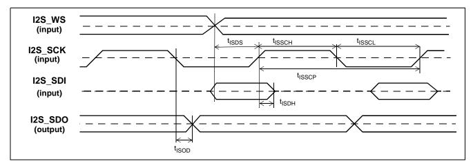
Figure 38 - Slave I<sup>2</sup>S Timing
