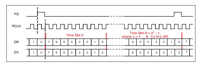
Figure 14 - TDM - PCM Master Functional Timing Diagram (8-bit, xeDX = 1)
