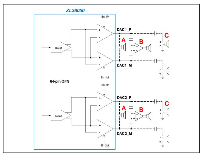
Figure 7 - Audio Output Configurations
