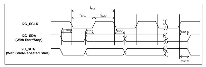
Figure 41 - I<sup>2</sup>C Timing Parameter Definitions
