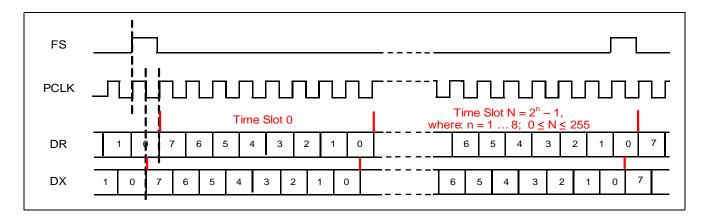
Figure 13 - TDM - PCM Master Functional Timing Diagram (8-bit, xeDX = 0)
