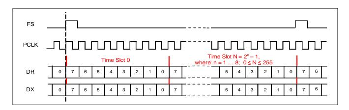
Figure 16 - TDM - GCI Master Functional Timing Diagram
