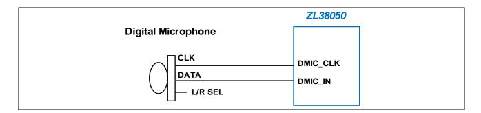
Figure 3 - Single Mono Digital Microphone Interface
