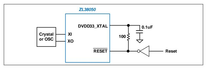
Figure 26 - Ultra-Low Power Operation Circuit
