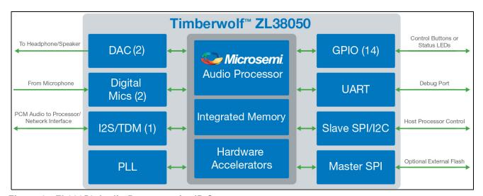
Figure 2 - ZL38050 Audio Processor for IP Cameras
