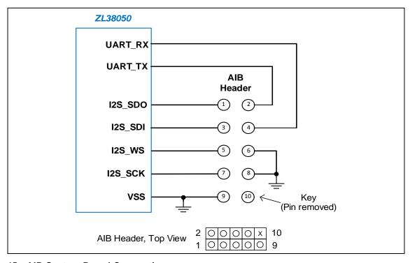
Figure 45 - AIB System Board Connection
