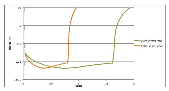
Figure 30 - THD+N Ratio versus  $V_{RMS}$  - Driving High Impedance
