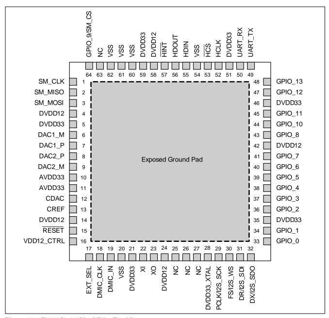
Figure 27 - ZL38050 64-Pin QFN - Top View
