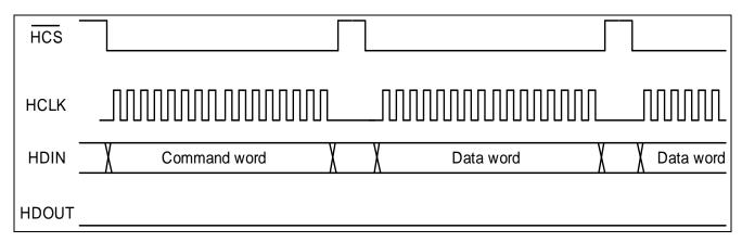
Figure 19 - SPI Slave Word Framing Mode - Write, Multiple Data Words
