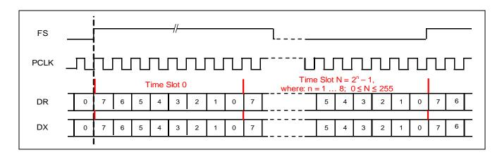
Figure 15 - TDM - GCI Slave Functional Timing Diagram
