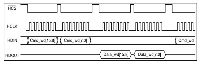
Figure 18 - SPI Slave Byte Framing Mode - Read
