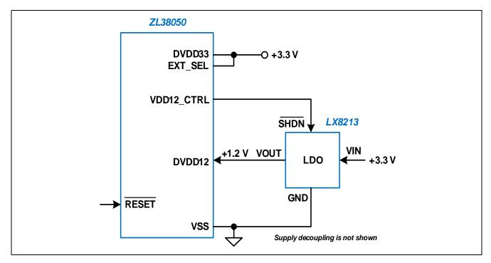
Figure 24 - External +1.2 V Power Supply Configuration
