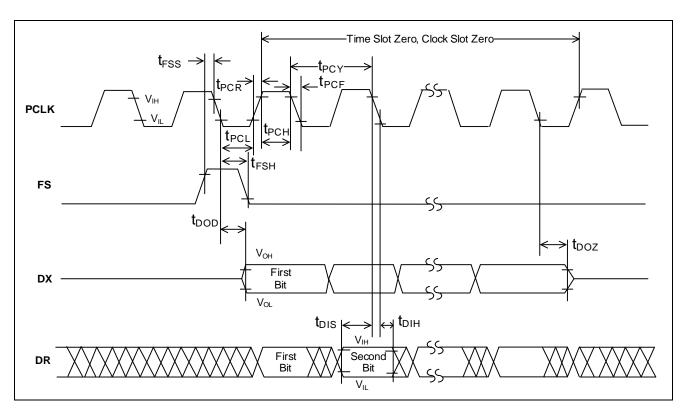
Figure 36 - PCM Timing, 8-bit with xeDX = 0 (Transmit on Negative PCLK Edge)
