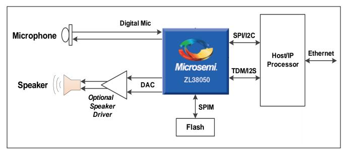
Figure 1 - IP Camera HD Voice 2-way Audio Application
