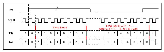
Figure 12 - TDM - PCM Slave Functional Timing Diagram (8-bit, xeDX = 1)
