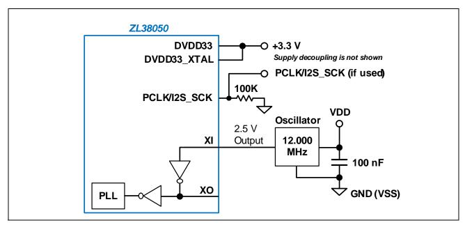
Figure 32 - Clock Oscillator Application Circuit
