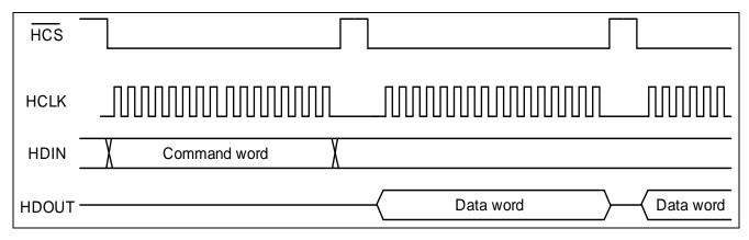
Figure 20 - SPI Slave Word Framing Mode - Read, Multiple Data Words
