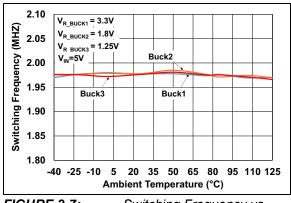
FIGURE 2-7: Switching Frequency vs. Temperature – Active Mode (LPM = Low, PWRHLD = High).
