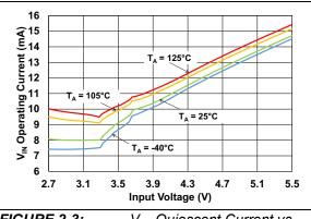
**FIGURE 2-3:**  $V_{IN}$  Quiescent Current vs. Input Voltage and Temperature – Active Mode (LPM = Low, PWRHLD = High).
