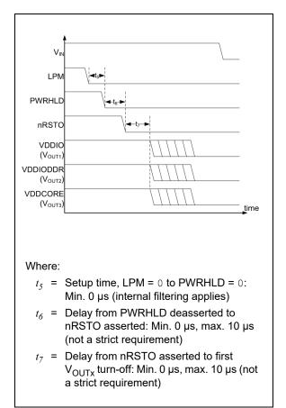
FIGURE 4-7: Power-Down (Shutdown) Sequence Timing Diagram.
