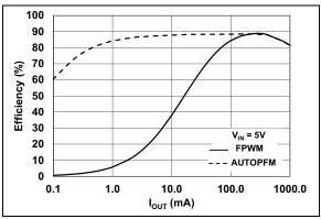
**FIGURE 2-5:** Buck2 Efficiency vs. Load Current Measured on PVIN2 (V<sub>OUT2</sub> = 1.2V).
