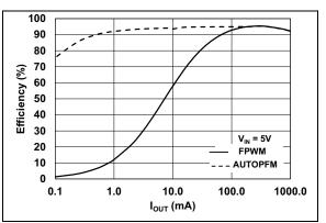
**FIGURE 2-4:** Buck1 Efficiency vs. Load Current Measured on PVIN1 (V<sub>OUT1</sub> = 3.3V).
