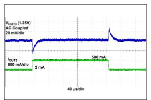
**FIGURE 2-16:** Buck3 Transient Response (Active Mode, V<sub>OUT3</sub> = 1.25V).
