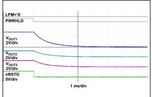
FIGURE 2-14: PWRHLD Shutdown Sequence.
