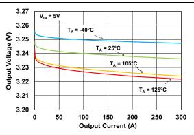
FIGURE 2-10: LDO Output Voltage vs. Output Current and Temperature (Load Regulation –  $V_{LOUT}$  = 3.3V).
