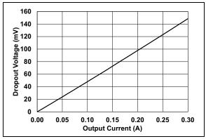
FIGURE 2-11: LDO Dropout Voltage vs. Load Current.
