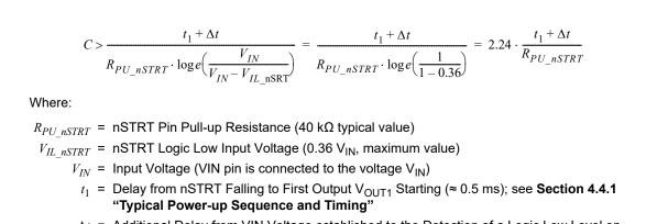
Δ*t* = Additional Delay from VIN Voltage established to the Detection of a Logic Low Level on nSTRT (due to internal logic wake-up time): ≈ 100 μs
