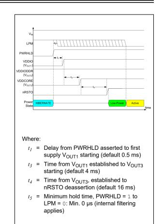
FIGURE 4-9: Start-up Sequence Exiting Hibernate Mode Timing Diagram.
