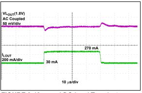
FIGURE 2-18: LDO Load Transient Response.
