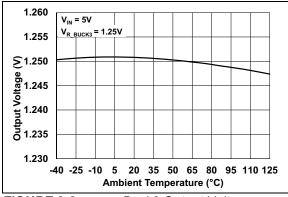
Buck3 Output Voltage vs. Temperature – V<sub>OUT3</sub> = 1.25V, Active Mode (LPM = Low, PWRHLD = High).
