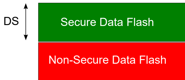
Figure 13-3. SAM L11 Data Flash Memory Mapping
