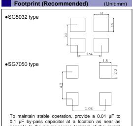
0.1  $\mu F$  by-pass capacitor at a location as near as possible to the power source terminal of the crystal product (between Vcc - GND).
