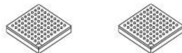
249 FOWLP 7.0mm x 7.0mm x 0.725mm, 0.4mm 间距 141 WLCSP 4.525mm x 4.525mm x 0.49mm, 0.35mm 间距
