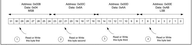
FIGURE 8-1: Accessing Multi-Byte Register Value.
