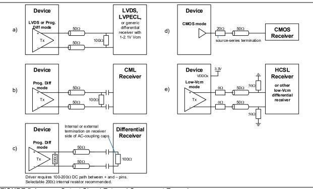
FIGURE 5-1: Output Signal External Component Examples.
