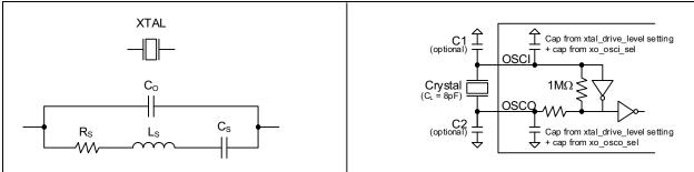
FIGURE 5-2: Crystal Equivalent Circuit/Recommended Crystal Circuit.
