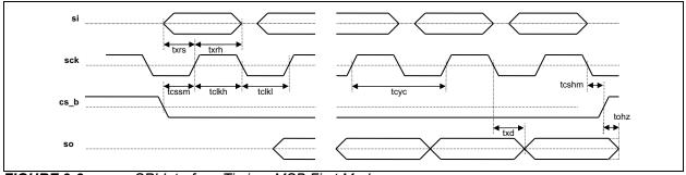
FIGURE 9-3: SPI Interface Timing, MSB First Mode.
