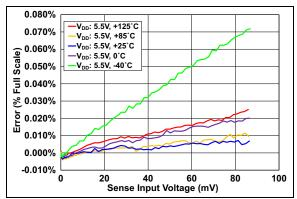
**FIGURE 2-5:** V<sub>SENSE</sub> Error vs. V<sub>SENSE</sub> Input Voltage at Multiple Temperatures.
