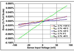
FIGURE 2-3: V<sub>SENSE</sub> Error vs. V<sub>SENSE</sub> Input Voltage, Bidirectional Mode.
