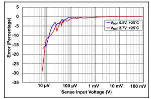
**FIGURE 2-1:** V<sub>SENSE</sub> Error vs. V<sub>SENSE</sub> Input Voltage.
