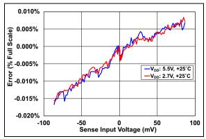
**FIGURE 2-4:** V<sub>SENSE</sub> Error vs. V<sub>SENSE</sub> Input Voltage, Bidirectional Mode.
