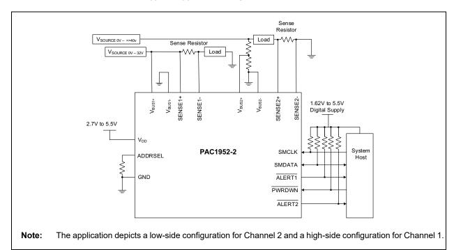
FIGURE 4-2: PAC195X-2 Low-Side Typical Application Diagram.
