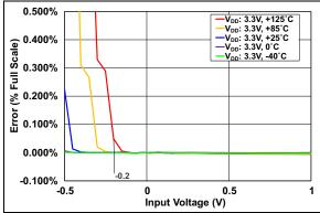
**FIGURE 2-15:** V<sub>BUS</sub> Error vs. V<sub>BUS</sub> Input Voltage at Multiple Temperatures (Bipolar Mode).
