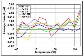
**FIGURE 2-28:** V<sub>BUS</sub> Input Leakage Current vs. Temperature and Common-Mode.
