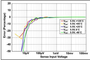
**FIGURE 2-7:** V<sub>SENSE</sub> Error vs. V<sub>SENSE</sub> Input Voltage at Multiple Temperatures.
