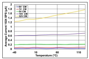
FIGURE 2-27: Average V<sub>SENSE</sub> Input Current – Active Mode, 1024 SPS vs. Temperature and Common-Mode.
