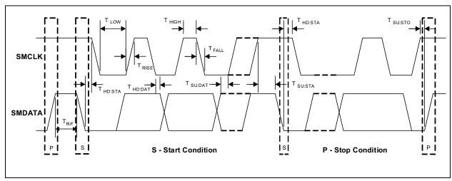
FIGURE 6-1: SMBus Timing Diagram.
