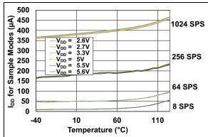
**FIGURE 2-23:** I<sub>DD</sub> vs.Temperature, Supply and Sample Rate.
