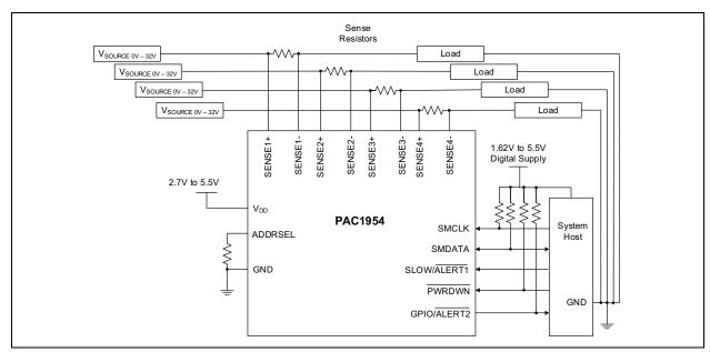
FIGURE 4-1: PAC195X-1 Typical Application Diagram.
