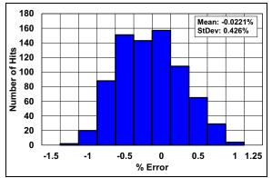
FIGURE 2-30: Clock Frequency Error -40°C to +125°C. Total Population 768 Devices.
