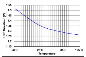
FIGURE 2-32: POR vs. Temperature.
