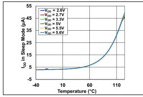
**FIGURE 2-24:** Sleep Mode Current vs. Temperature and Supply.
