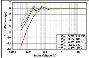
**FIGURE 2-12:** V<sub>BUS</sub> Error vs. V<sub>BUS</sub> Input Voltage at Multiple Temperatures.
