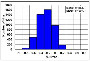
FIGURE 2-31: Clock Frequency Error at +30°C. Total Population 4,723 Devices.
