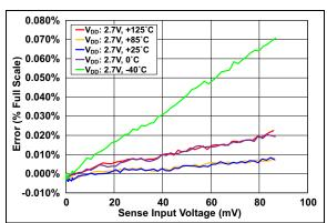
**FIGURE 2-6:** V<sub>SENSE</sub> Error vs. V<sub>SENSE</sub> Input Voltage at Multiple Temperatures.
