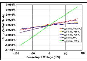
**FIGURE 2-2:** V<sub>SENSE</sub> Error vs. V<sub>SENSE</sub> Input Voltage, Bidirectional Mode.
