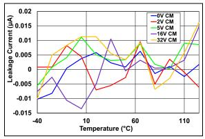
**FIGURE 2-26:** V<sub>SENSE</sub> Input Leakage Current vs. Temperature and Common-Mode.
