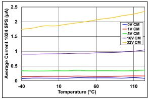
**FIGURE 2-29:** V<sub>BUS</sub> Input Current – Active Mode, 1024 SPS vs. Temperature and Common-Mode.
