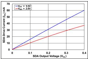
**FIGURE 2-20:** SDA Drive Current vs. V<sub>OL</sub> at +25°C.
