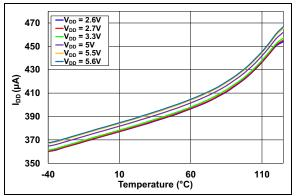
**FIGURE 2-21:**  $I_{DD}$  vs. Temperature and Supply at 1024 SPS.
