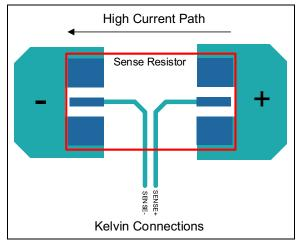
FIGURE 4-3: PCB Pattern for Sense Resistor.
