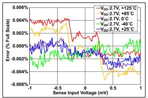
**FIGURE 2-10:** V<sub>SENSE</sub> Error vs. V<sub>SENSE</sub> Input Voltage, Bidirectional Mode (Zoom View).
