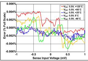
**FIGURE 2-9:**  $V_{SENSE}$  Error vs.  $V_{SENSE}$  Input Voltage, Bidirectional Mode (Zoom View).
