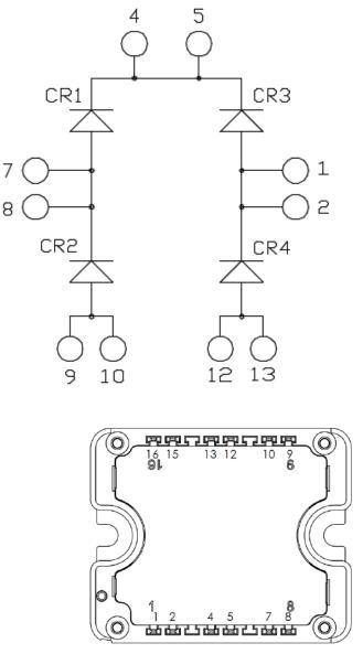
All multiple inputs and outputs must be shorted together 1/2; 7/8; 9/10; 12/13
