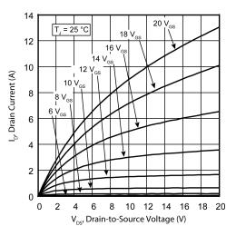
Figure 2 • Drain Current vs. V<sub>DS</sub>
