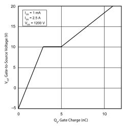
Figure 6 • Gate Charge Characteristics
