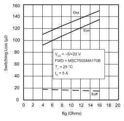
Figure 13 • Switching Energy vs. Rg
