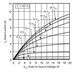
Figure 3 • Drain Current vs. V<sub>DS</sub>
