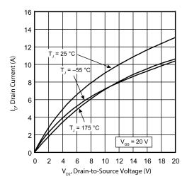
Figure 1 • Drain Current vs. V<sub>DS</sub>
