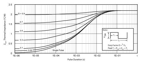
Figure 17 • Maximum Transient Thermal Impedance
