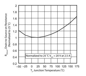
Figure 5 • RDS(on) vs. Junction Temperature
