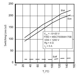
Figure 14 • Switching Energy vs. Temperature
