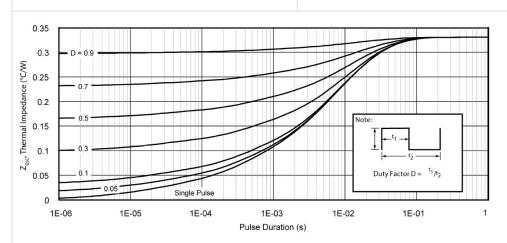
Figure 20 • Maximum Transient Thermal Impedance
