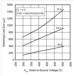
Figure 15 • Switching Energy Eon vs.  $\mathbf{V}_{\mathrm{DS}}$  and  $\mathbf{I}_{\mathrm{D}}$
