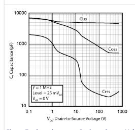
Figure 7 ● Capacitance vs. Drain-to-Source Voltage | Figure 8 ● I<sub>D</sub> vs. Gate-to-Source Voltage
