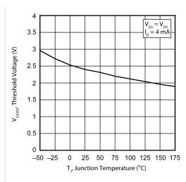
Figure 18 • Threshold Voltage vs. Junction Temp.
