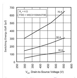
Figure 12 • Switching Energy Eoff vs.  $\mathbf{V}_{DS}$  and  $\mathbf{I}_{D}$
