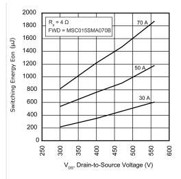
Figure 11  $\bullet$  Switching Energy Eon vs.  $V_{DS}$  and  $I_{D}$
