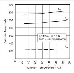
Figure 14 • Switching Energy vs. Temperature
