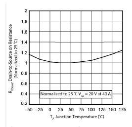
Figure 5 ● R<sub>DS(on)</sub> vs. Junction Temperature
