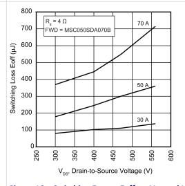
Figure 16 • Switching Energy Eoff vs. V<sub>DS</sub> and I<sub>D</sub>
