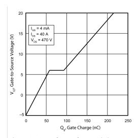
Figure 6 • Gate Charge Characteristics
