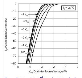
Figure 9 ● I<sub>D</sub> vs. V<sub>DS</sub> 3<sup>rd</sup> Quadrant Conduction
