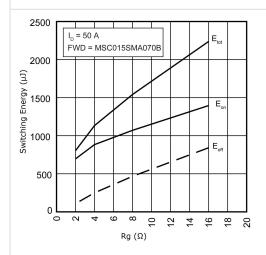
Figure 13 • Switching Energy vs. R<sub>g</sub>
