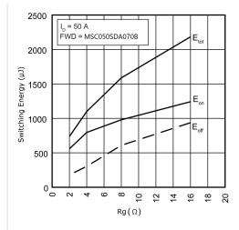
Figure 17 • Switching Energy vs. R<sub>g</sub>
