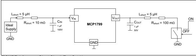
FIGURE 4-2: Short Circuit Test Set-Up.
