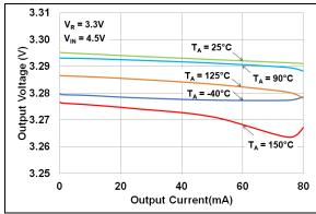
**FIGURE 2-3:** Output Voltage vs. Output Current ( $V_R = 3.3V$ ).
