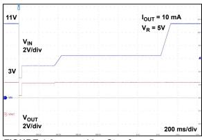
FIGURE 4-3: Line Step from Dropout.
