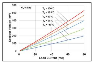
**FIGURE 2-5:** Dropout Voltage vs. Output Current.
