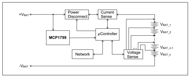
FIGURE 6-1: Smart Battery Pack Application Example.
