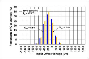
**FIGURE 2-1:** Input Offset Voltage Histogram.
