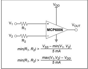
FIGURE 4-2: Protecting the Analog Inputs.
