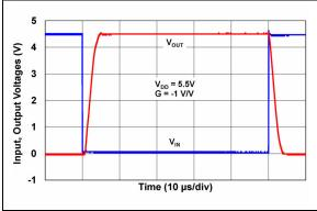
FIGURE 2-36: Large Signal Inverting Pulse Response.
