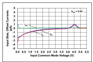
**FIGURE 2-7:** Input Bias, Offset Current vs. Common-Mode Voltage.
