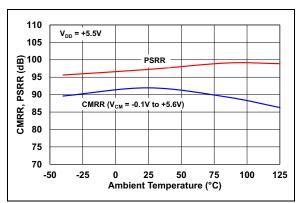
FIGURE 2-9: CMRR, PSRR vs. Ambient Temperature.
