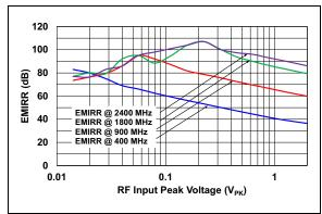
**FIGURE 2-24:** EMIRR vs. RF Input Peak-to-Peak Voltage.
