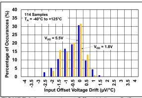
**FIGURE 2-2:** Input Offset Voltage Drift Histogram.
