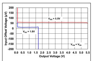
**FIGURE 2-5:** Input Offset Voltage vs. Output Voltage.
