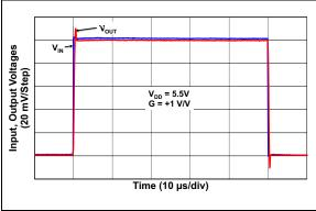
FIGURE 2-33: Small Signal Noninverting Pulse Response.
