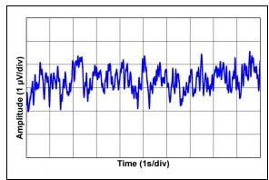
FIGURE 2-31: 0.1 Hz to 10 Hz Voltage Noise.
