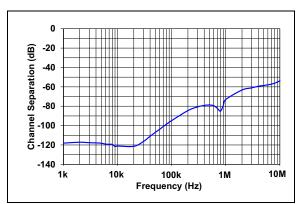
FIGURE 2-25: Channel Separation vs. Frequency.
