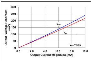
FIGURE 2-17: Output Voltage Headroom vs. Output Current.
