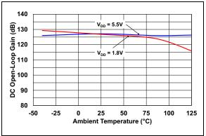
**FIGURE 2-10:** DC Open-Loop Gain vs. Ambient Temperature.
