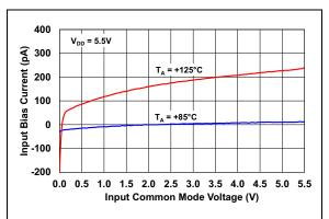
FIGURE 2-8: Input Bias Current vs. Common-Mode Input Voltage.
