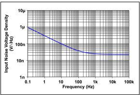
FIGURE 2-28: Input Noise Voltage Density vs. Frequency.
