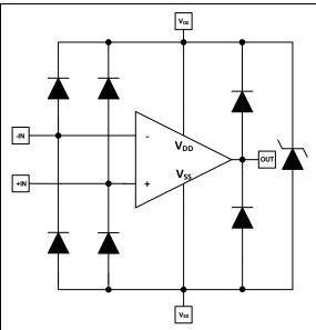
FIGURE 4-1: Simplified Analog Input ESD Structures.
