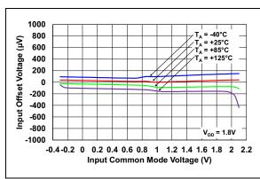
FIGURE 2-3: Input Offset Voltage vs. Common-Mode Input Voltage.
