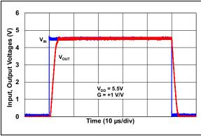
**FIGURE 2-35:** Large Signal Noninverting Pulse Response.
