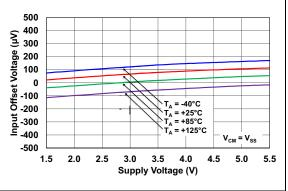
**FIGURE 2-6:** Input Offset Voltage vs. Power Supply Voltage.
