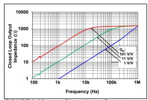
**FIGURE 2-22:** Closed-Loop Output Impedance vs. Frequency.
