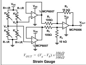
FIGURE 4-10: Pressure Sensor Amplifier.
