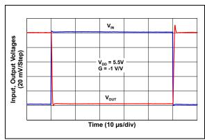
FIGURE 2-34: Small Signal Inverting Pulse Response.
