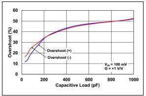
**FIGURE 2-39:** Overshoot vs. Capacitive Load.
