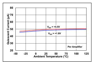
**FIGURE 2-12:** Quiescent Current vs. Ambient Temperature.
