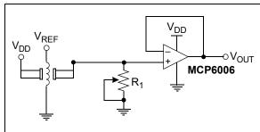
FIGURE 4-9: CO Gas Sensor Circuit.
