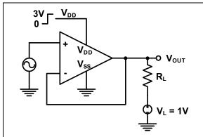
FIGURE 4-3: Start-up Test Circuit.
