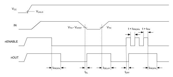
Figure 5. SGM896A/SGM898A Timing Diagram
