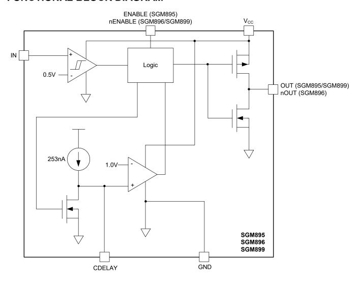
Figure 2. SGM895/SGM896/SGM899 Block Diagram
