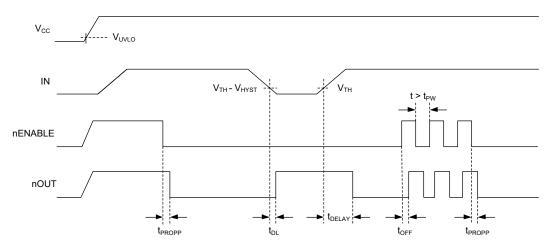
Figure 6. SGM896P/SGM898P Timing Diagram
