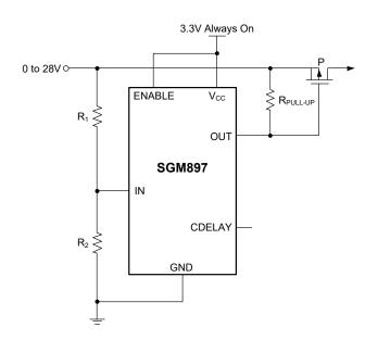
Figure 9. Over-Voltage Protection
