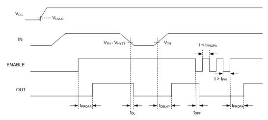
Figure 3. SGM895A/SGM897A Timing Diagram
