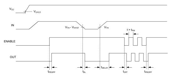
Figure 4. SGM895P/SGM897P Timing Diagram
