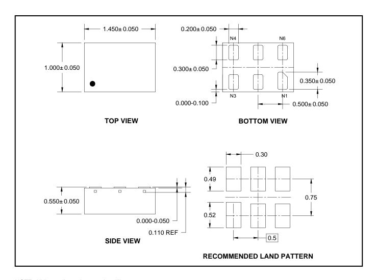
NOTE: All linear dimensions are in millimeters.
