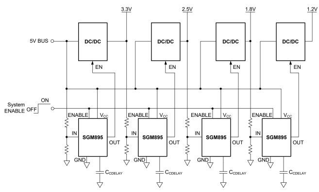
Figure 11. Multiple-Output Sequencing
