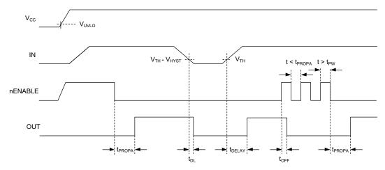
Figure 7. SGM899A Timing Diagram
