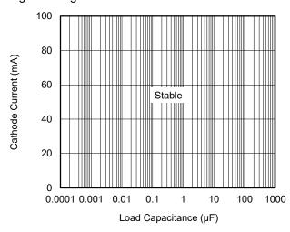
Figure 6. Cathode Current vs. Load Capacitance
