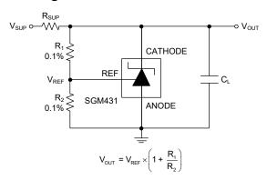
Figure 5. Shunt Regulator Schematic
