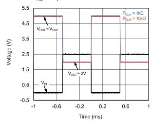
Figure 4. Output Response with Various Cathode Current
