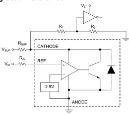
Figure 3. Comparator Application Schematic
