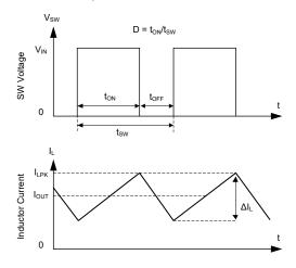
Figure 3. Converter Switching Waveforms in CCM
