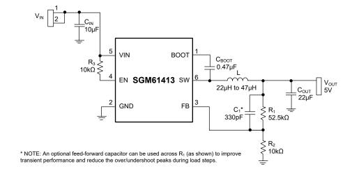
Figure 7. Typical Application Circuit
