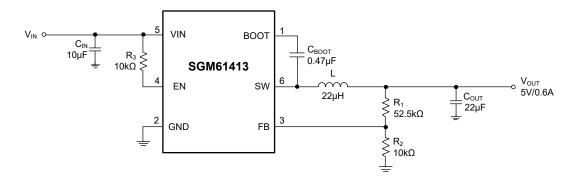
Figure 4. 5V Output Typical Application Circuit
