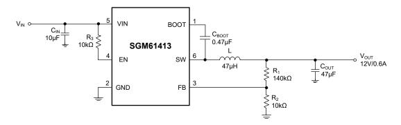
Figure 5. 12V Output Typical Application Circuit
