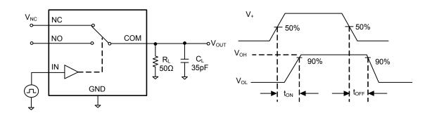
Test Circuit 2. Switching Times  $(t_{\text{ON}},\,t_{\text{OFF}})$
