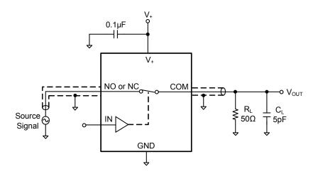
Test Circuit 6. -3dB Bandwidth
