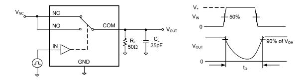
Test Circuit 3. Break-Before-Make Time Delay (t<sub>D</sub>)
