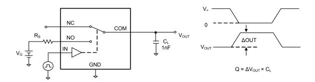
Test Circuit 7. Charge Injection (Q)
