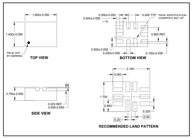
NOTE: All linear dimensions are in millimeters.
