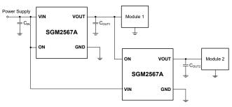
Figure 7. Power Supply Sequencing without a GPIO Input
