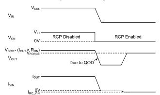
NOTES:  $V_{\text{SRC}}$  is the input power supply to the equipment.  $V_{\text{FORCE}}$  is the external power source forced at VOUT pin.  $I_{\text{VIN}}$  is the current of VIN pin.  $I_{\text{OUT}}$  is output load current.
