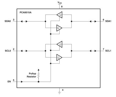
Figure 2. Logic Diagram (Positive Logic)
