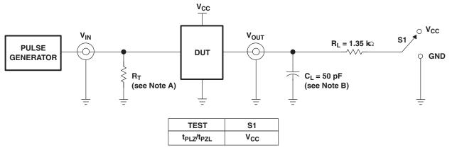
TEST CIRCUIT FOR OPEN-DRAIN OUTPUT
