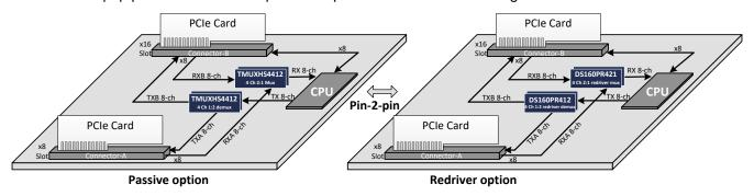
Figure 8-2. Pin-to-pin passive vs redriver option for PCIe lane switching
