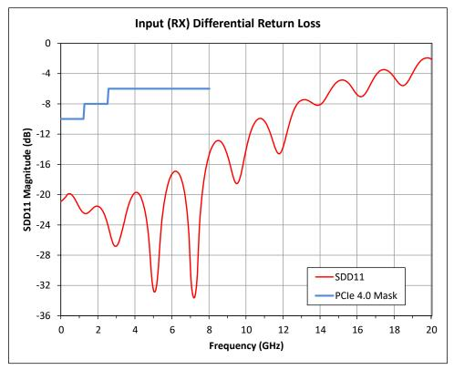
Figure 6-3. Typical RX Differential Return Loss
