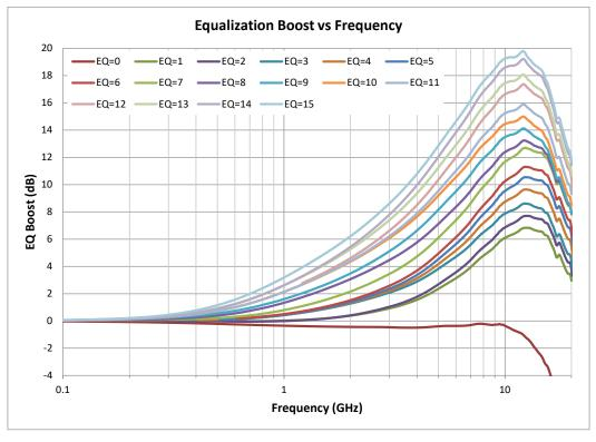
Figure 6-1. Typical EQ Boost vs Frequency
