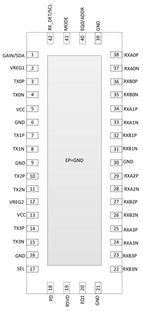
Figure 5-1. RUA Package 42-Pin WQFN Top View
