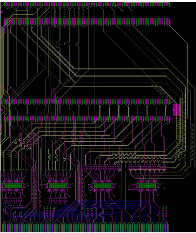
Figure 11-2. Layout example for PCIe lane muxing application
