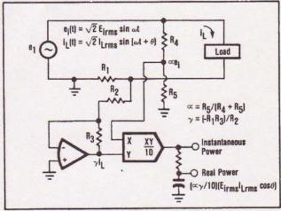
FIGURE 11. Single-Phase Instantaneous and Real Power Measurement.
