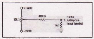
FIGURE 2. Optional Trimming Configuration.
