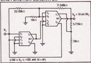
FIGURE 10. Sine Function Generator.
