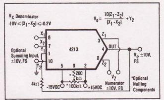
FIGURE 4. Divider Connection.
