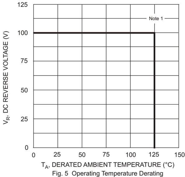
Note 1: Part mounted on FR-4 board with recommended pad layout, which can be found on our website at <http://www.diodes.com/datasheets/ap02001.pdf>.
