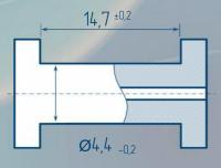
5000 turns, wire Ø0,063 mm coil resistance 620
