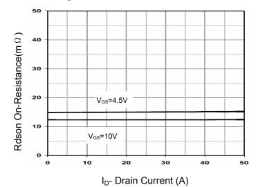
Figure 3 Rdson- Drain Current
