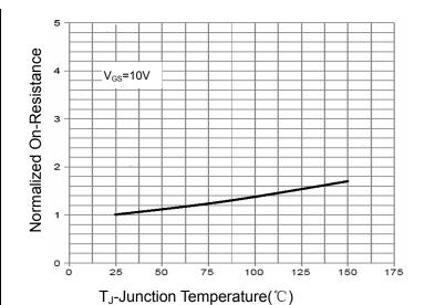
**Figure 4 Rdson-Junction Temperature**
