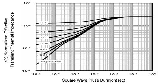
**Figure 11 Normalized Maximum Transient Thermal Impedance**
