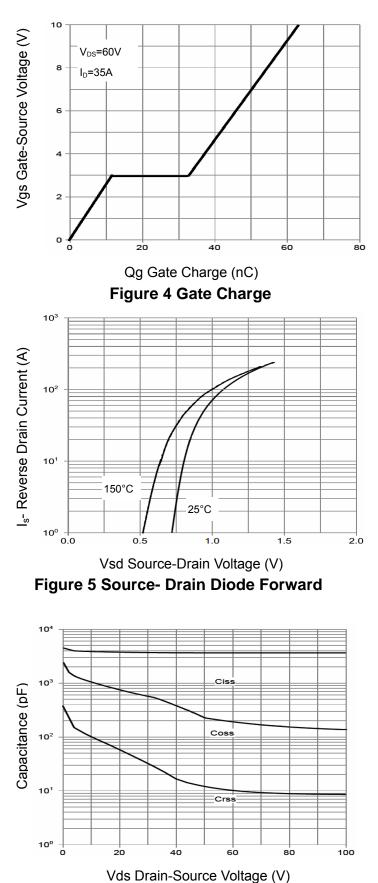
Figure 6 Capacitance vs Vds
