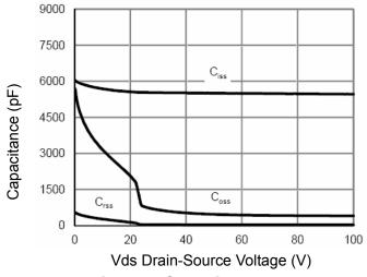
Figure 7 Capacitance vs Vds
