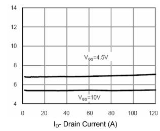
Figure 3 Rdson- Drain Current
