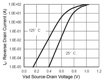
Figure 6 Source- Drain Diode Forward
