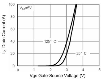
**Figure 2 Transfer Characteristics**
