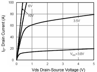
**Figure 1 Output Characteristics**
