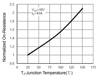
**Figure 4 Rdson-Junction Temperature**
