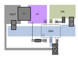
Figure 4. Recommended PCB Layout Diagram
