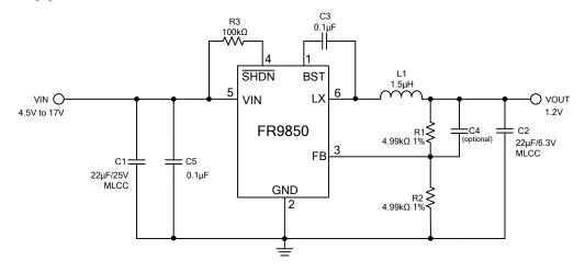
Figure 2.  $C_{\text{IN}}/C_{\text{OUT}}$  use Ceramic Capacitors Application Circuit
