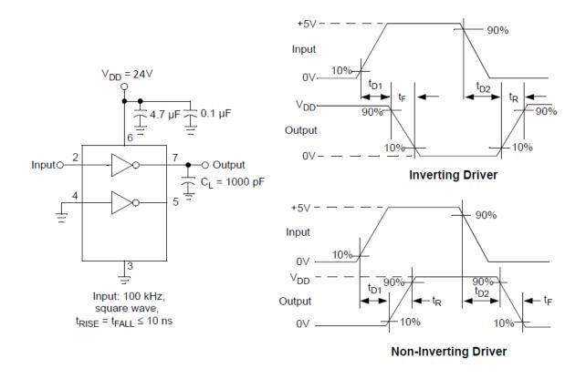
Figure 3.1 Switching Time Test Circuit
