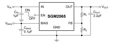
**Figure 1. Typical Application Circuit**
