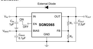
Figure 4. Reverse Protection Reference Design
