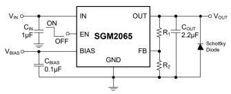
Figure 5. Negatively Biased Output Application
