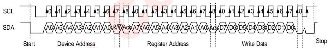
Fig 26 I 2 C Write Timing
