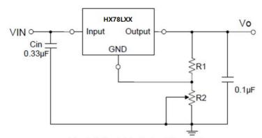
Fig.3 Adjustable Output Regulator
