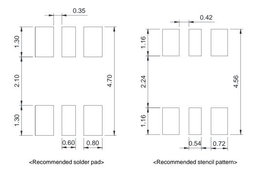
It recommended that metal mask is designed to be under 80% of dimension of solder pad.
