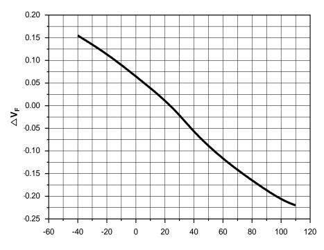
$\triangle V_F = V_F - V_F(25^{\circ}C)$  Junction Temperature [°C]
