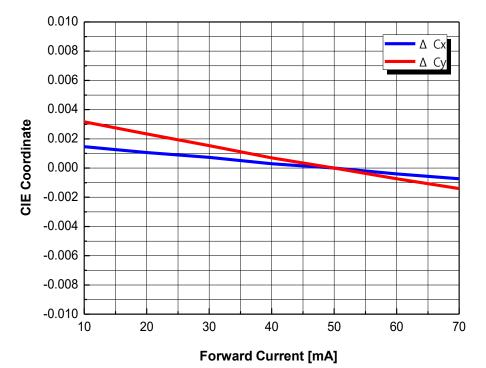
Fig 5. Forward Current vs. CIE X, Y Shift, T<sub>j</sub> = 25°C
