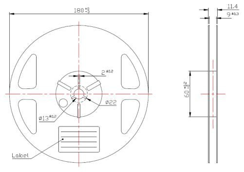
( Tolerance:  $\pm 0.2,\ Unit:\ mm$  )
