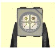
(3) When populating boards in SMT production, there are basically no restrictions regarding the form of the pick and place nozzle, except that mechanical pressure on the surface of the resin must be prevented. This is assured by choosing a pick and place nozzle which is larger than the LED's reflector area.
