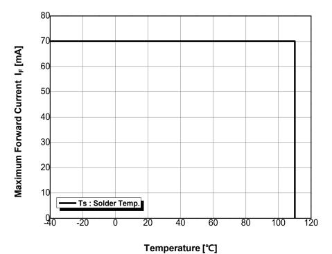
Fig 9. Maximum Forward Current vs. Temperature
