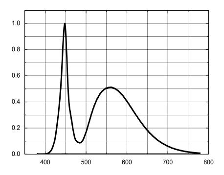
Fig 1. Color Spectrum,  $I_F$  = 50mA,  $T_j$  = 25°C, RH30%
