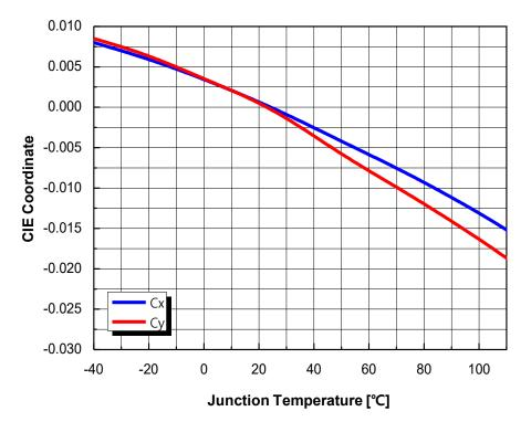
Fig 8. Chromaticity Coordinate vs. Junction Temperature,  $I_F = 50 \text{mA}$
