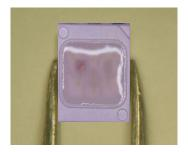
These conditions must be considered during the handling of such devices. Compared to standard encapsulants, silicone is generally softer, and the surface is more likely to attract dust. As mentioned previously, the increased sensitivity to dust requires special care during processing. In cases where a minimal level of dirt and dust particles cannot be guaranteed, a suitable cleaning
