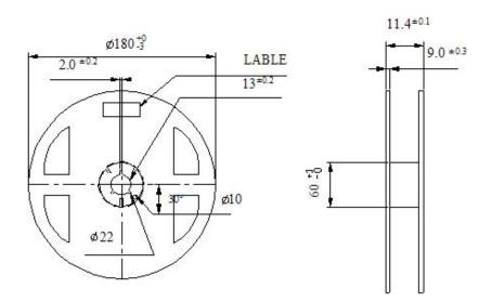
(Tolerance:  $\pm 0.2$ , Unit: mm)
