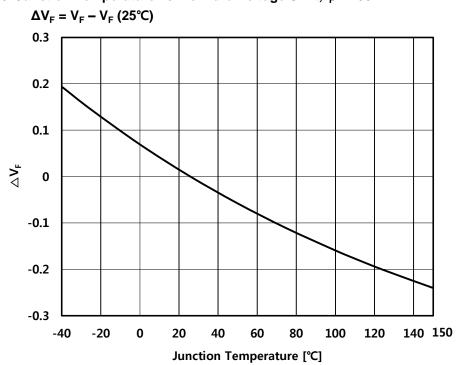
Fig 6. Junction Temperature vs. Forward Voltage Shift, I<sub>F</sub> = 150mA
