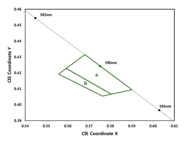
Fig 10. Color Coordinate Diagram,  $T_a = 25^{\circ}C$ ,  $I_F = 150mA$
