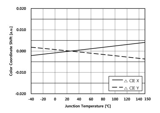
Fig 8. Junction Temperature vs. Color Coordinate Shift,  $I_{F}$ = 150mA
