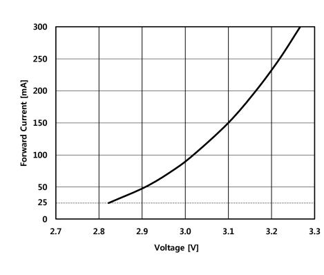
Fig 3. Forward Voltage vs. Forward Current,  $T_a = 25^{\circ}C$
