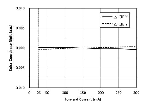
Fig 5. Forward Current vs. Color Coordinate Shift,  $T_a = 25^{\circ}C$
