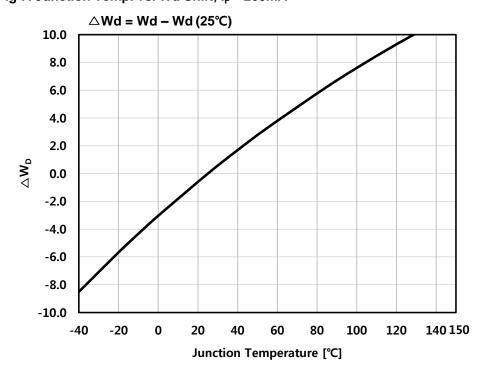
Fig 8. Relative Forward vs. Junction Temperature, I<sub>F</sub> = 200mA
