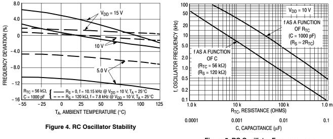
Figure 5. RC Oscillator Frequency as a Function of R<sub>tc</sub> and C<sub>tc</sub>
