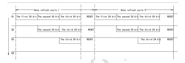
Chip cascade, data transmission and retransmission procedure: Data (D1) is sent from controller. When chip 1 finishes receiving the first 24bit, chip 1 does not retransmit data (D2) still and controller continues to send data, chip 1 receives the second 24bit. As the first 24 bit is existed in chip1, chip 1 retransmits the second 24bit out through DO. Chip 2 receives the data (D2) retransmitted from Chip1. At this time, chip 2 still does not retransmit data
