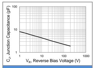
Fig.2 Typical Junction Capacitance
