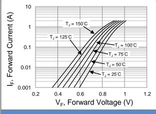
Fig.4 Typical Forward Characteristics
