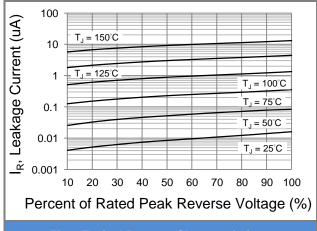
Fig.3 Typical Reverse Characteristics
