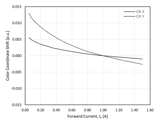
Fig 5. Forward Current vs. Color Coordinate Shift,  $T_a = 25^{\circ}C$
