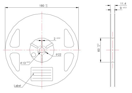
(Tolerance:  $\pm$ 0.2, Unit: mm)
