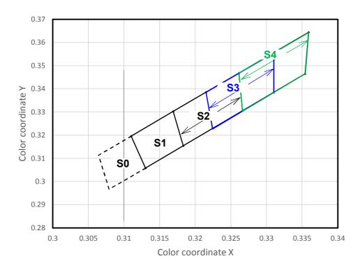
Fig 10. Color Coordinate Diagram,  $T_a = 25^{\circ}C$ ,  $I_F = 1.0A$
