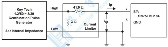
Figure 16. Overvoltage-Stress Test Circuit
