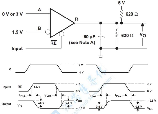
NOTE A: This value includes probe and jig capacitance (± 10%).
