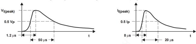
Figure 15. Short-Circuit Current Waveforms
