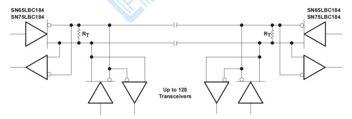
NOTE A: The line should be terminated at both ends in its characteristic impedance (RT = ZO). Stub lengths off the main line should be kept as short as possible.
