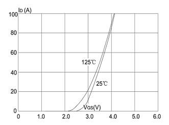
**Figure 2: Typical Transfer Characteristics**
