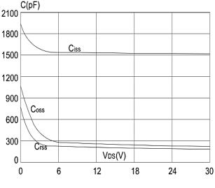
**Figure 6: Capacitance Characteristics**
