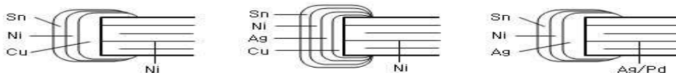
(Inner Electrode : Ni Type I) (Inner Electrode : Ni Type II) (Inner Electrode : Ag/pd Type)
