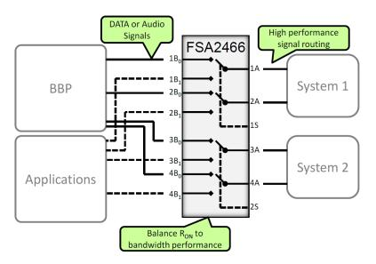
Figure 1. Typical Mobile Phone Application
