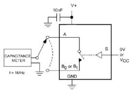
Figure 7. On / Off Capacitance Measurement Setup
