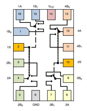
Figure 2. FSA2466UMX (Top View)
