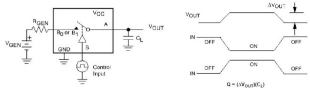
Figure 6. Charge Injection
