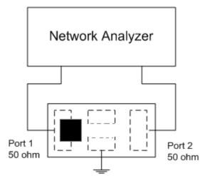
Test Instrument: Agilent E5071C Network Analyzer or equivalent.
