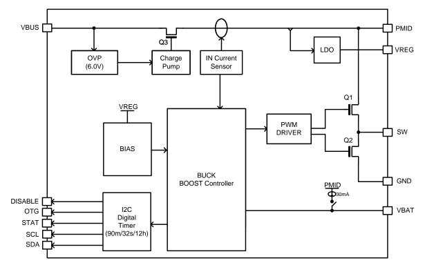
Figure 2: IC and System Block Diagram
