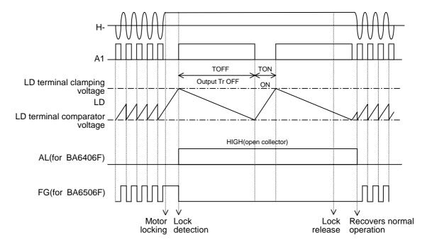
Fig.10 Lock protection (CR timer system) timing chart
