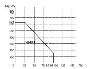
\* Reduce by 6.24 mW/°C over 25°C. (70.0mm x 70.0mm x 1.6mm glass epoxy board)
