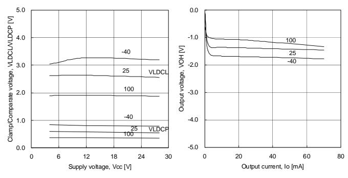
Fig.7 Clamp-comparison voltage of capacitor for lock detection
