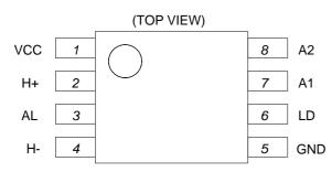
Fig.1 Pin configuration
