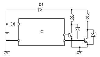
Fig.14 Separation of a power supply line
