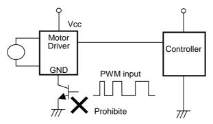
Fig.16 GND Line PWM switching prohibited
