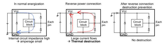
Fig.13 Current flow when power is connected reversely
