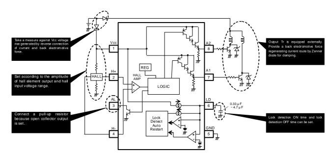
Fig.9 application circuit
