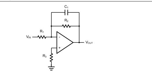
Figure 5. Low Pass Active Filter
