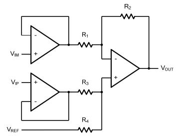
Figure 6. Instrument Amplifier
