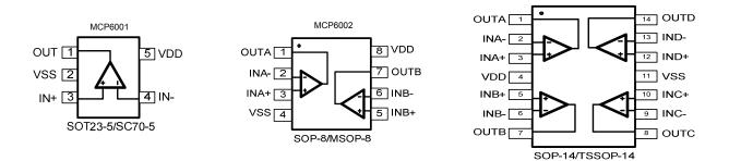
Figure 1. Pin Assignment Diagram
