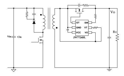
Figure B: JW7726BL Typical Application for high-side.
