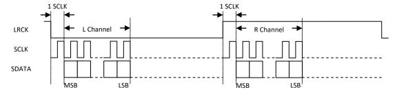
Figure 2a I<sup>2</sup>S Serial Audio Data Format
