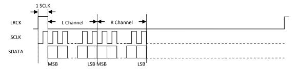
Figure 2c DSP/PCM Mode A Serial Audio Data Format
