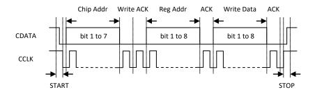
Figure 1a I<sup>2</sup>C Write Timing
