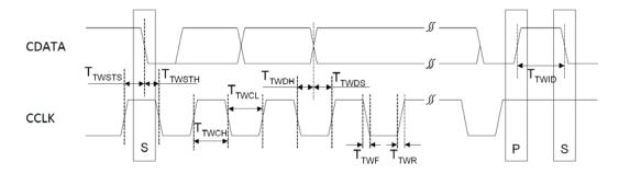
Figure 3 I<sup>2</sup>C Timing
