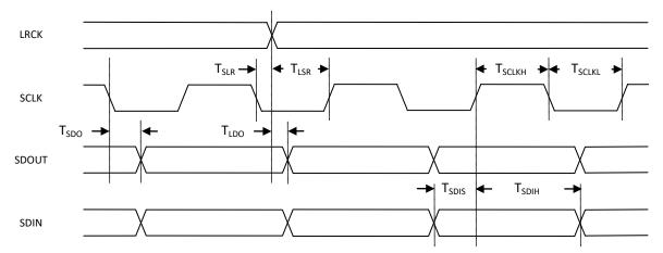
Figure 4 Serial Audio Port Timing
