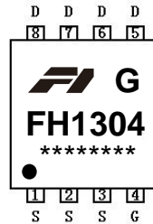
Marking and pin Assignment
